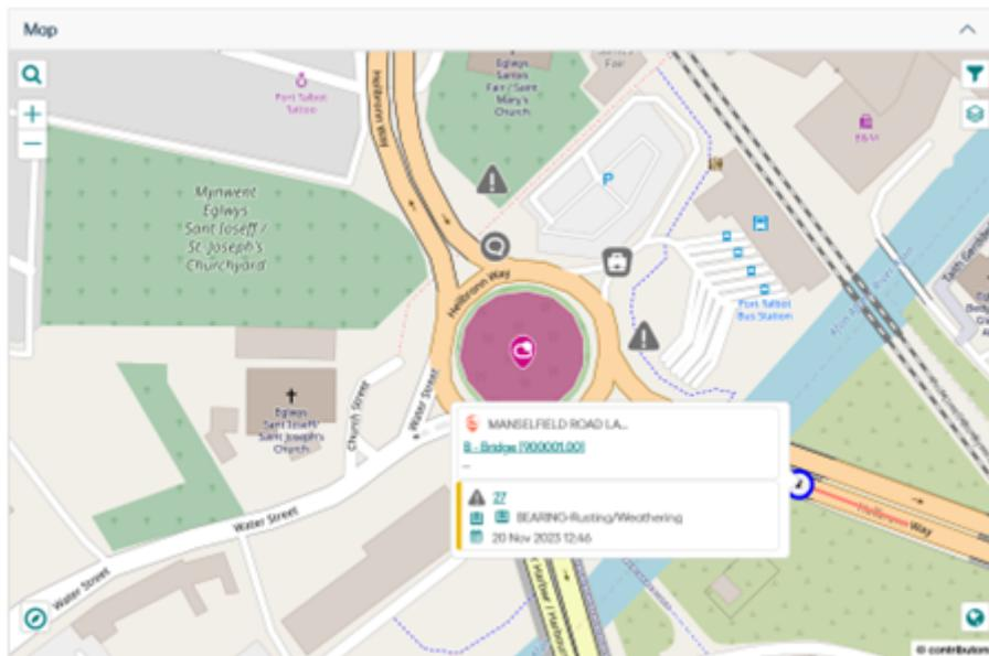
For example, here we can see the Defect does not have its own spatial geometry so it is shown with its Feature.
