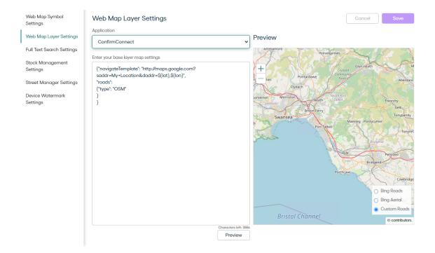
**Note:** The page removes the need to request SQL from Confirm to apply these settings. It will ensure that the entered text is within the database limit of 4000 characters and will use simple parsing to validate JSON text.
