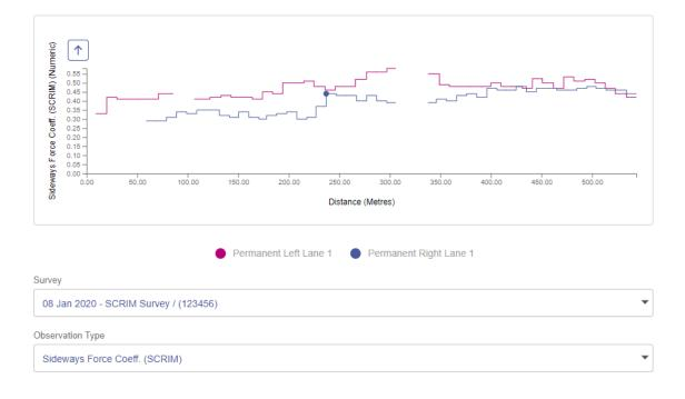
This component lists Surveys for the current Linear Feature which have a Start Date. If there are Observations available they are grouped by their Cross Sectional Position and plotted on a chart along the length of the Feature.
